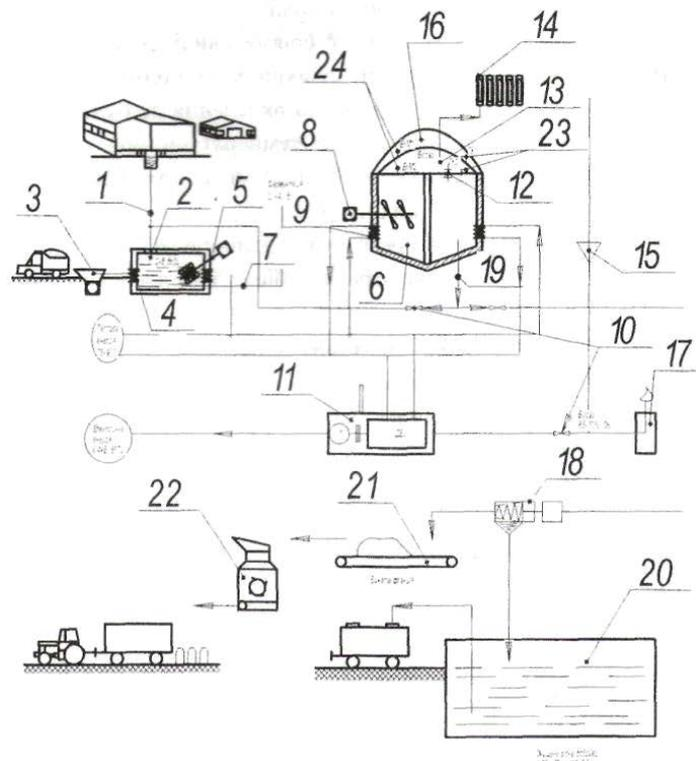
**Picture 1 The scheme of production line of biomass into gas and biological organic fertilizers**
