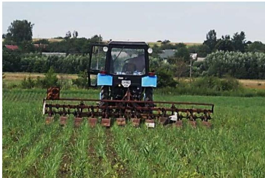
**Fig. 3. Switchgrass cultivation between rows with cultivator SF - 5.4 aggregated to the tractor MTZ-82**
